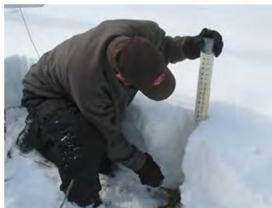
Obtaining snow depth and core sample
