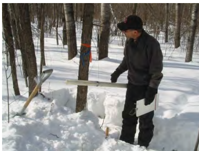
Establish base weight of empty sampling tube
