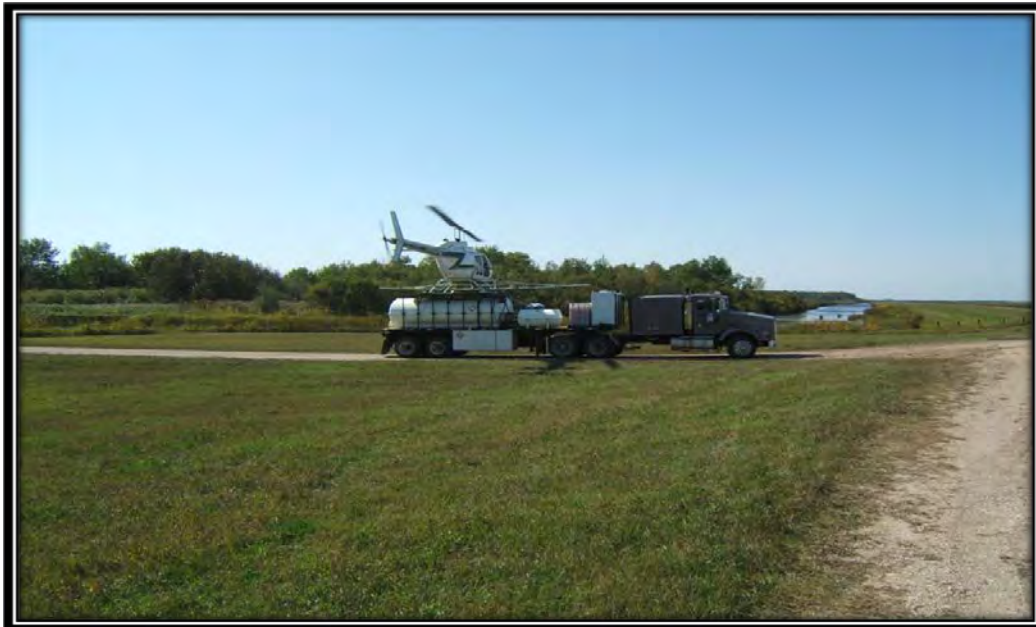
Spray helicopter landing on support truck to refill with chemical and also to refuel.
