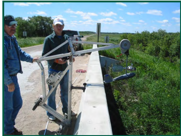
Measuring flow with bridge crane
